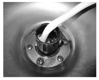
The small holes line up with the holes and the three large screws are refitted.
