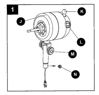
• Slide the fan motor assembly (J) onto the upper pole aligning the screw holes of both. Re-insert and tighten the locking screw (N).
